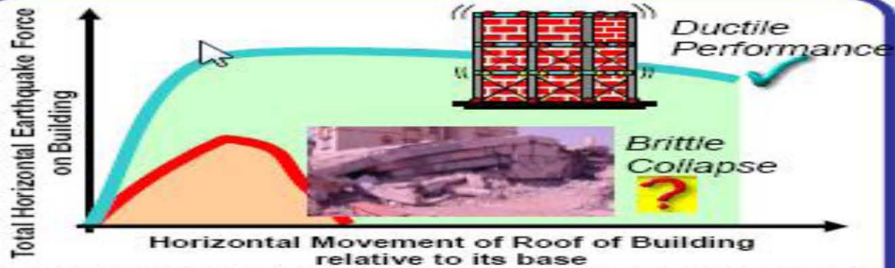
(a) Building performances during earthquakes: two extremes – the ductile and the brittle.
